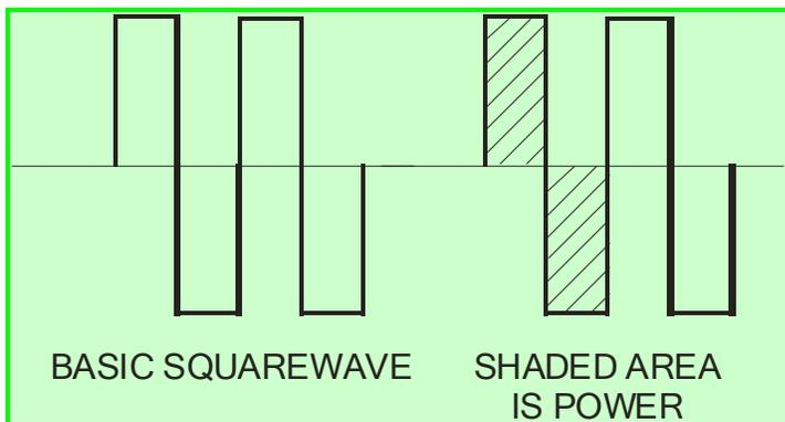
The area under the squarewave represents power and if one compares this with a sinewave at the same frequency, then it is obvious that the area under a sinewave is much less than the square wave.
