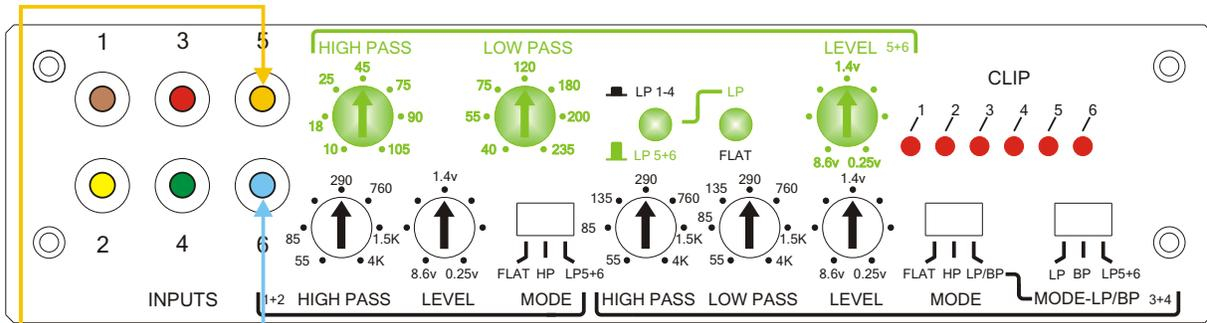
THESE TWO INPUTS MAY BE Y-ADAPTED AND THE CHANNELS RUN IN BRIDGE MODE
