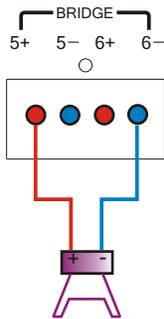
Chs 5+6 MAY BE RUN IN BRIDGE MODE (MIN SPEAKER IMPEDANCE IS 4 OHMS)
