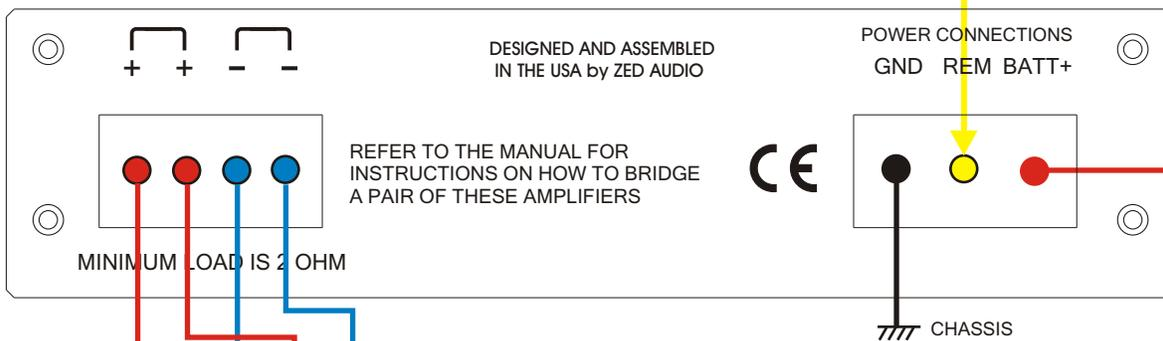
A SECOND DRIVER MAY BE CONNECTED IN PARALLEL WITH THE FIRST DRIVER THE NET MINIMUM LOAD IS 2 OHMS SO USE TWO 4 OHM DRIVERS. (1,000w)
