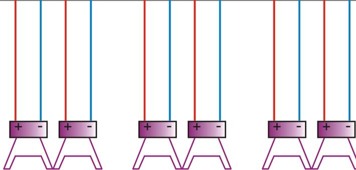
ANY PAIR OF CHANNELS MAY BE BRIDGED (MIN SPEAKER IMPEDANCE IS 4 OHMS)
