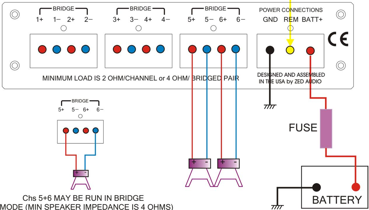
Chs 5+6 MAY BE RUN IN BRIDGE MODE (MIN SPEAKER IMPEDANCE IS 4 OHMS)
