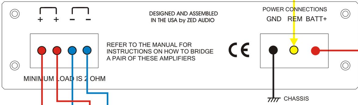
A SECOND DRIVER MAY BE CONNECTED IN PARALLEL WITH THE FIRST DRIVER THE NET MINIMUM LOAD IS 2 OHMS SO USE TWO 4 OHM DRIVERS. (1,000w)
