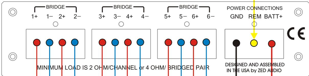
MINIMUM LOAD IS 2 OHM/CHANNEL or 4 OHM/ BRIDGED PAIR
