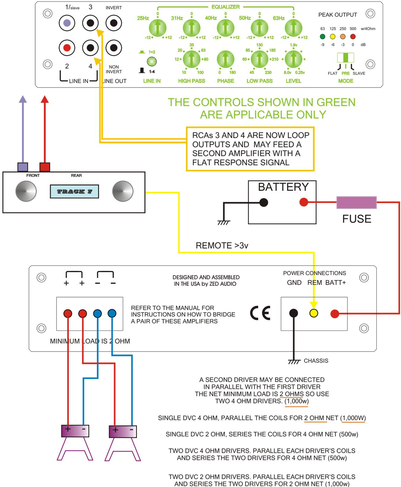
**MINOTAUR** driving one or more speakers as a stand alone amplifier from a four output signal source and set to **FLAT** mode. This drawing applies to any configuration where a single **MINOTAUR** is used.
