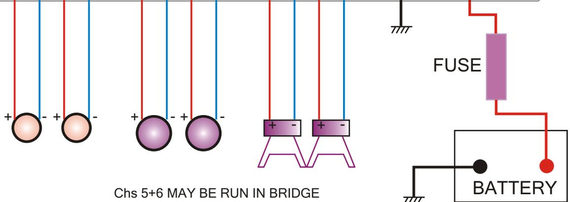
Chs 5+6 MAY BE RUN IN BRIDGE MODE (MIN SPEAKER IMPEDANCE IS 4 OHMS)
